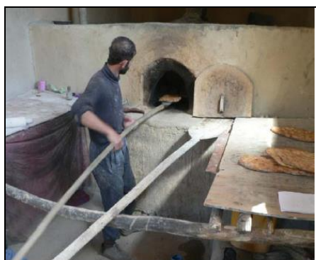
Figure 4: Dash oven fired by coal in a community bakery in Afghanistan (HELVETAS Swiss Intercooperation Afghanistan)
