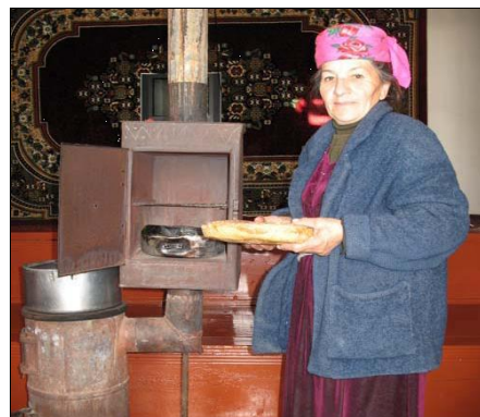
Figure 6: Double-walled chimney bread oven in a house in Tajikistan (Afghanistan Energy)
