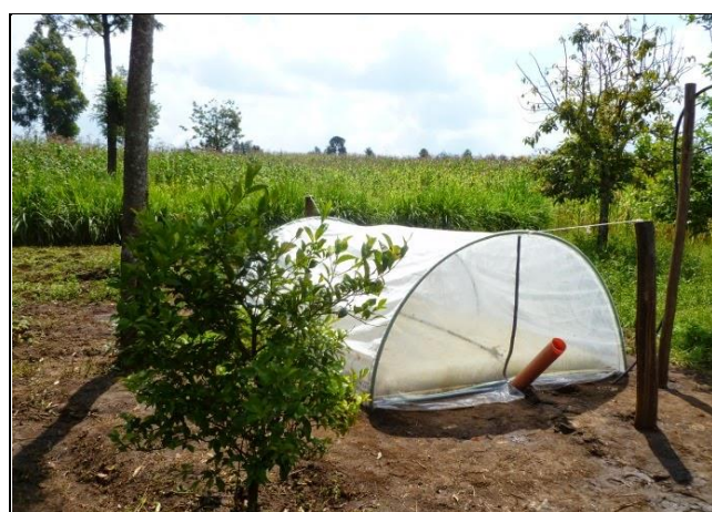
Figure 7: Flexi-biogas system developed by Biogas International requiring 20-30 kg of dung per day to produce biogas ( www.biogas.co.ke )
